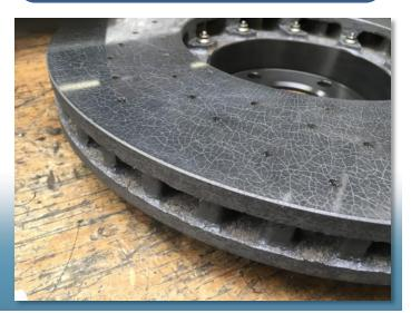
B) CCM: with HIGH content of carbon fibers, baseline recommendation RSC 2
